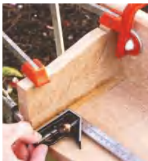
STEP 19. Glue a bracket to each end piece and cramp them together. Check for centrality
